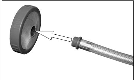
3. Replace the fitted inlet connector with the inlet connector supplied.
