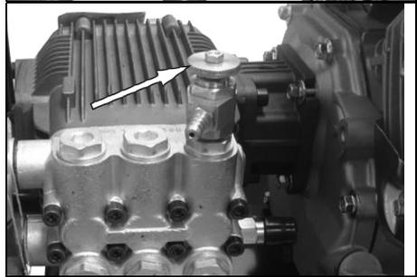
7. When the water spray being ejected is consistent and at high pressure close the self suction valve.
